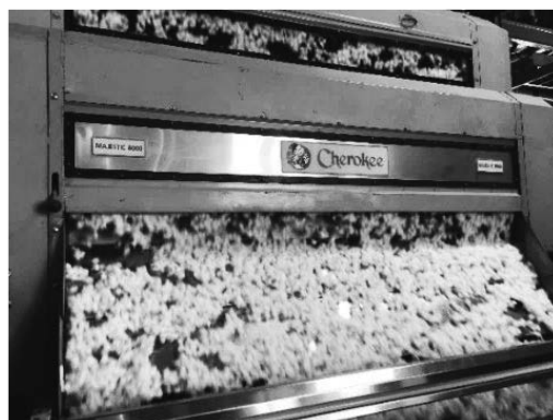
Figure 4.2 Ginning (automatic cotton ginning machine)
