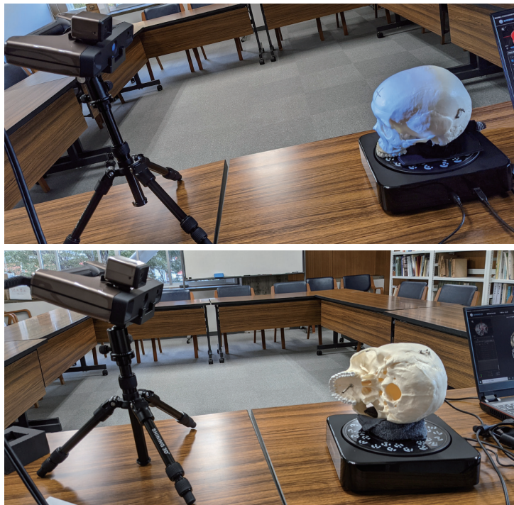
Figure 2. Settings for 3D scanning for Einscan scanner. The target object is the anatomical model and the angle is 1 and 2 in Figure 3.
